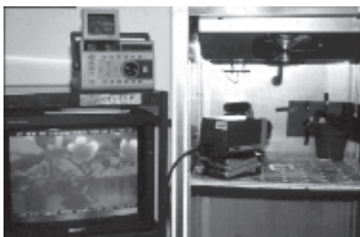
Figure 1. Use of infrared thermography to study freezing in plants. Infrared camera (Inframetrics Model 760 Infrared Radiometer) is set up inside an environmental chamber along with a potted strawberry plant. Control unit sitting on top of a video monitor is used to adjust the camera parameters while the experiment is in progress. The entire experiment is videotaped for future evaluation.
